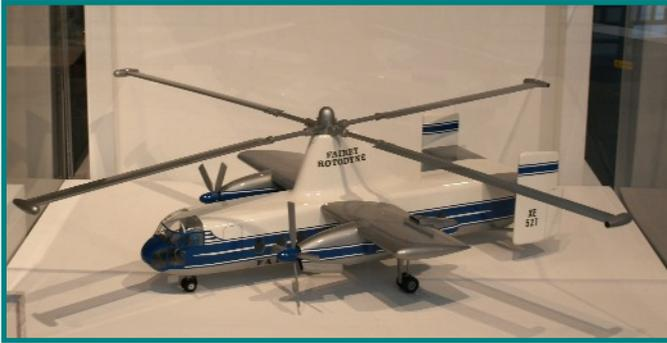
**Model of the Fairey Rotodyne, a 1950s VTOL aircraft which took off as a helicopter, but functioned as an autogyro during flight. Performance was satisfactory but the project failed commercially in 1962. Its technological successor, the Bell-Boeing Osprey, did not enter service until 2005.**
