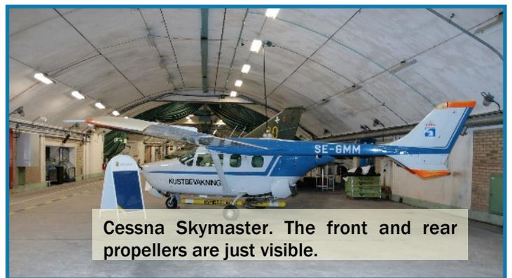
Cessna Skymaster. The front and rear propellers are just visible.
